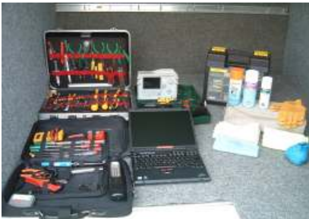
Equiped for the job ( NoteBook, Signal meter. Lead kit, toolbox & tool pad)
